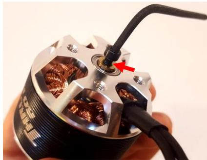
Apply Loctite to the retaining bolt
