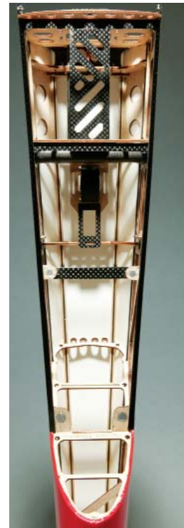
Composite laminate bulkhead shows carbon fiber exterior wall and end of longitudinal carbon tubes at bottom.
