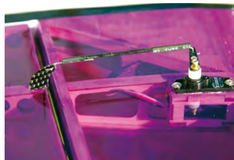
The control horns are carbon fibre and if you are into it and want more, try a set of carbon fibre servo arms. They provide increased throw and strength.
