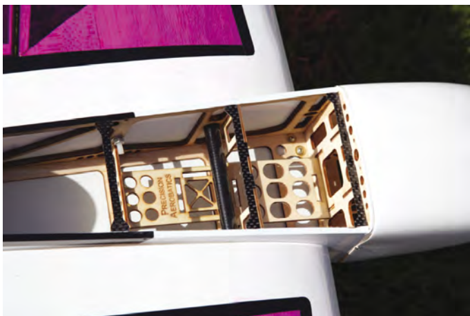
C.N.C. cut parts and plenty of carbon fibre throughout.
