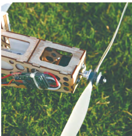
A choice of fire-wall or stick motor mounts are included.
