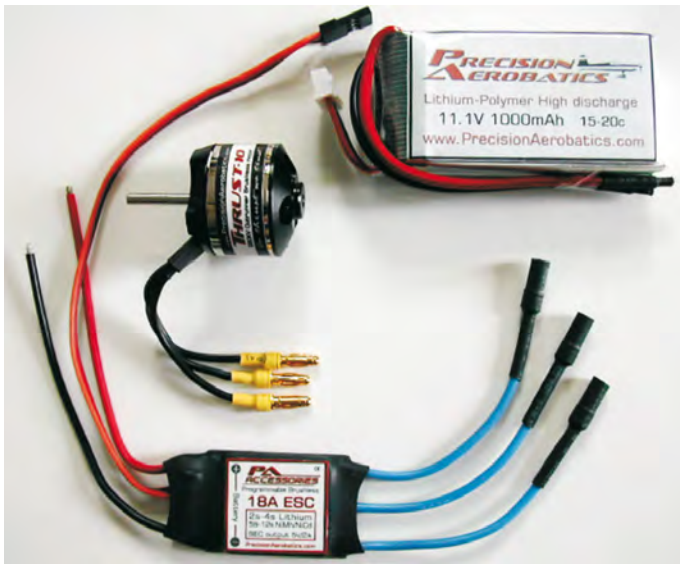
The Precision Aerobatics power setup consists of PA Thrust 10™ 930kv outrunner motor, PA 3S LiPo 1000mAh 15-20c battery pack, Electronic Speed control: PA 18A programmable brushless, Hyperion 6ch receiver with four BMS 306B Bluebird servo. With an APC 10X4.7 SF Power output: 900g of Thrust
