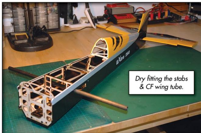
Horizontal Stab in place and a spot-on alignment.
