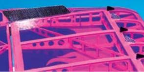
The carbon fiber side-force generators and vortex generators aid in high-alpha and knife-edge flight.
