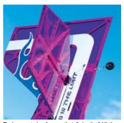
The huge control surfaces on the tail give the Addiction fiber main spar and dual alignment XL its awesome 3D capabilities. Also, You can see the dowels with a plastic thumbscrew high quality construction trough the covering.
