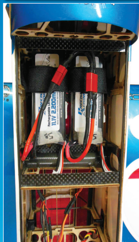
Batteries easily fit behind the firewall to balance out the Addiction XL.
