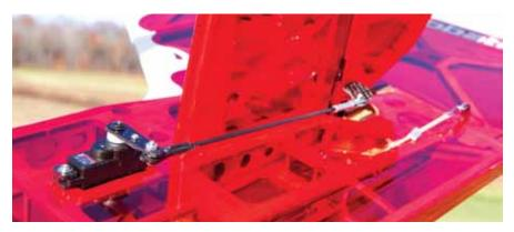
The hardware includes German-made ball links and CNC-machined clevises.
