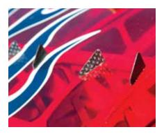
The Addiction X came with these wingmounted, carbon-fiber vortex generators
