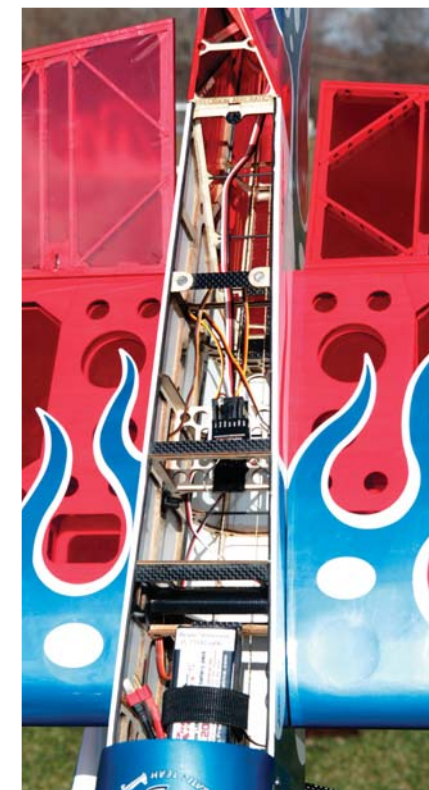
The secret to the Addiction X's feather-light and super-rigid airframe is the carbon fiber reinforced airframe.
