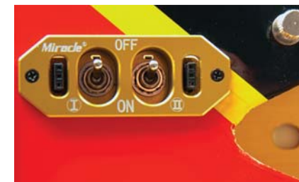
The B&E Graphix Miracle Switch professionally controls power for both the radio and ignition.
