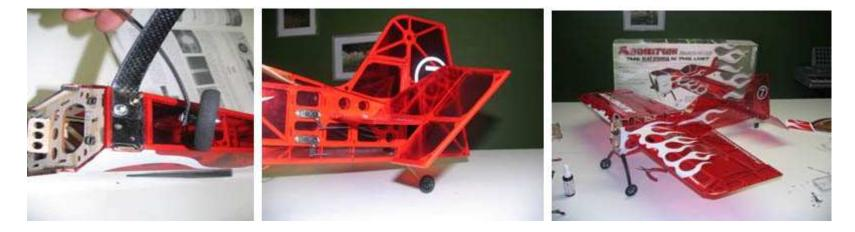
Time to concentrate on the business end. The motor cage is already done and is very well engineered. Fibre fusion at its best on the motor mounting plate( is that what its called). Install the Thrust 20 but don't forget to remove the C clip or there will be friction.
