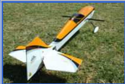
Removable wings with CF tube
