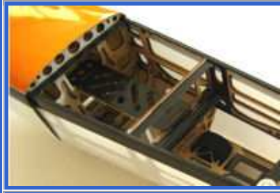
CF Battery Tray plenty of space for batteries up to 11.1V 2200 mah
