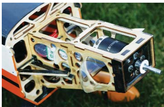
Two scoops direct a lot of cooling airflow over the motor to keep it running at peak efficiency.
