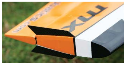
The carbon fiber vortex generators smooth the airflow over the wing tip and noticeably reduce wing rock during high alpha maneuvers.
