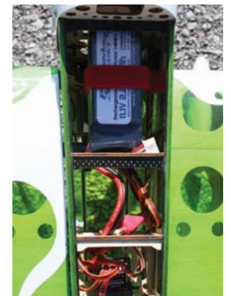
Access to the battery, onboard RC equipment and wing attachment is under the Addiction's canopy.
