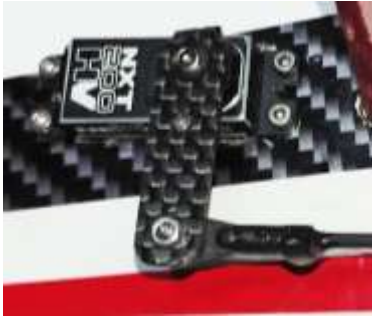
CF Elevator servo arm – Note: Ball link underneath the servo arm
