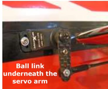
CF CNC machined elevator servo arm
