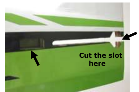
Stabilizer slot and Elevator Servo Opening
