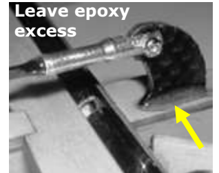
Aileron control horn
