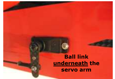
CF CNC machined rudder servo arm
