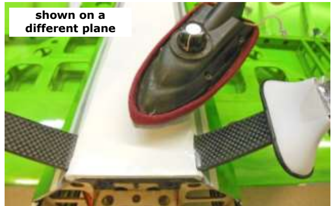
Apply covering over the LG bay
