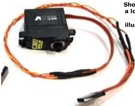
PA Lightweight servo extension
