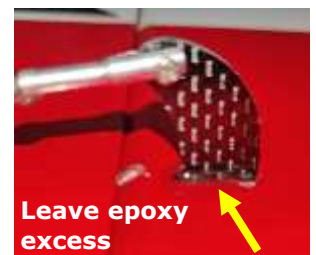
Aileron control horn
