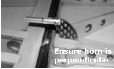
Test fit control horn
