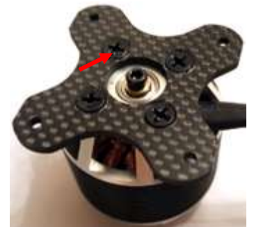
Bolts head must NOT protrude
