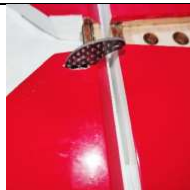
CF CNC machined elevator servo arm
