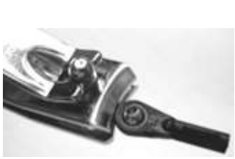
Trim the tab off the ball link
