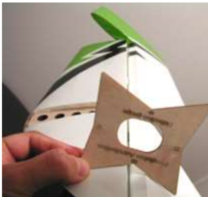
Deflect the elevator to approx 55° to set the hinge gap
