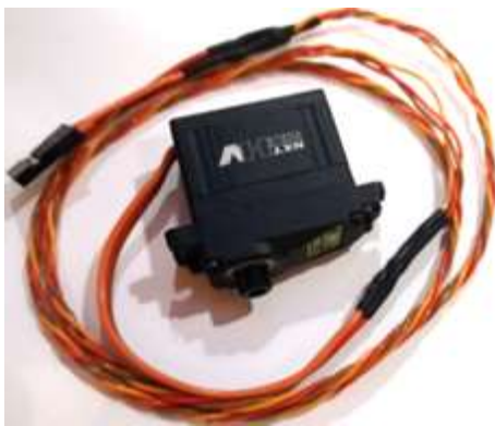
PA Lightweight servo extension
