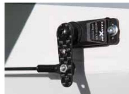
The precision hardware package has ball links that make the connections between the servo arm and control surface very solid.
