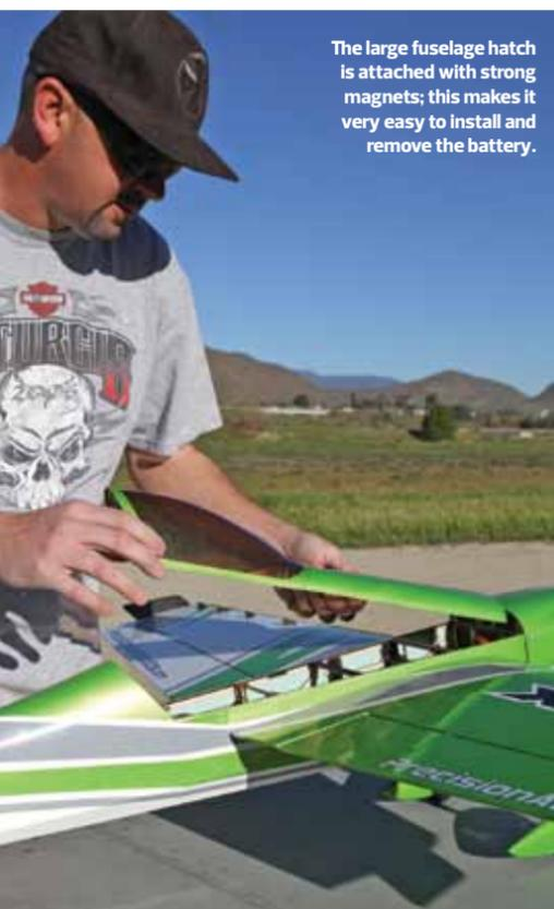
The large fuselage hatch is attached with strong magnets; this makes it very easy to install and remove the battery.
