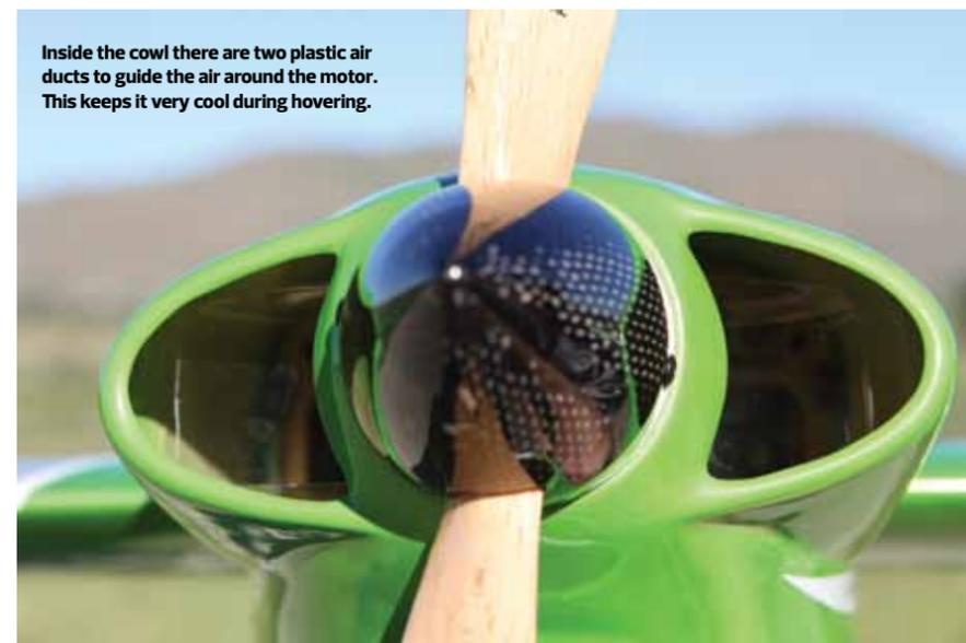
Inside the cowl there are two plastic air ducts to guide the air around the motor. This keeps it very cool during hovering.
