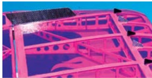
The carbon fiber side-force generators and vortex generators aid in high-alpha and knife-edge flight.
