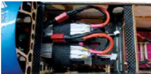
Two 3-cell 2200mAh LiPo battery packs are used to power the Addiction XL. This is a great setup because many modelers, like myself, use 2200mAh batteries in other models so it is nice not needing custom packs.
