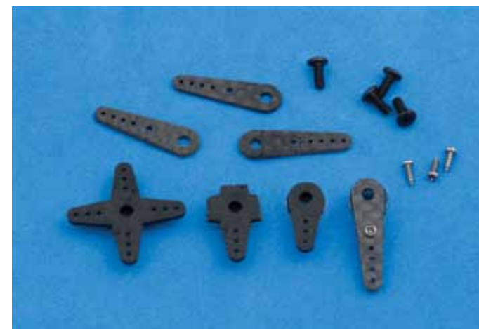
The steps to complete the servo horns are all shown in this one photo. First, cut off the three un-needed arms, then sand off the rough edges, and screw the carbon arm to the plastic arm.
