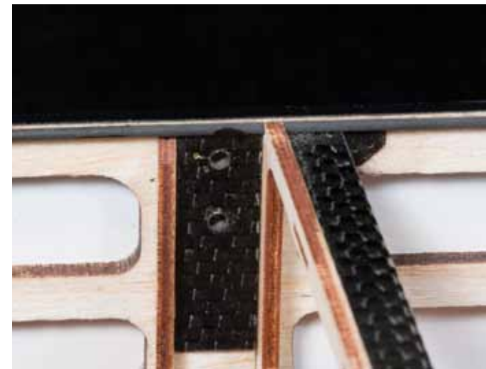
An example of the FiberFusion® construction approach is this reinforced area of the fuselage, where the upper wing cabane attaches.
