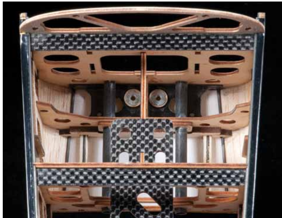
This top view into the forward end of the fuselage demonstrates the thought and engineering that went into the FiberFusion® design approach, strategically using carbon and wood for the strongest, stiffest and lightest structure possible.
