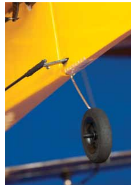
▲ The tail wheel is sturdy and very simple. Just epoxy it into the rudder and put a piece of reinforced packing tape over it for extra security!
