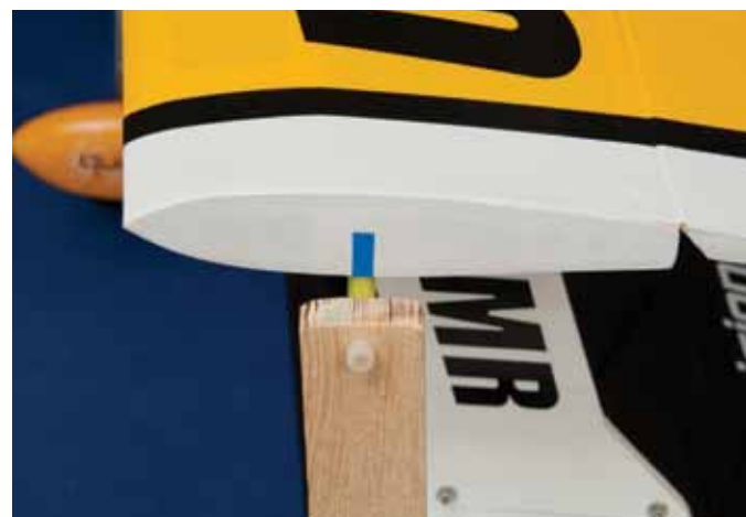
▲ This close-up shows how the upper wing rests on the CG tool that I built to balance the model, per the recommendations in the instruction manual. I used a plastic bolt with a piece of tygon tubing slid over it, to assure slip-free contact with the wing.
