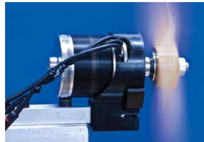
This photo shows the Thrust 40 motor in action, during a bench test to evaluate performance characteristics with different propellers.
