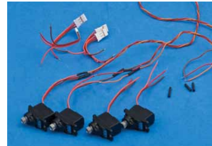
This demonstrates the steps involved in splicing in the servo extension wire. By taking this approach vs. using pre-made servo extensions, several grams of weight are saved. This step takes some time, but is not difficult to do.
