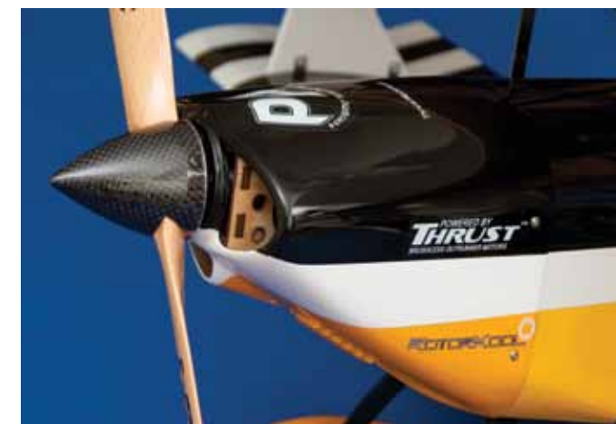
The cowl fits perfectly and lines up nicely with the spinner, as well as the plastic cooling scoops that direct air onto the rotating case of the Thrust 40 outrunner motor.
