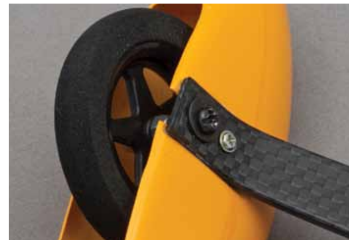
The landing gear hardware goes together smoothly. I put a drop of medium CA glue into the space between the wheel pant and landing gear, to prevent rotation.
