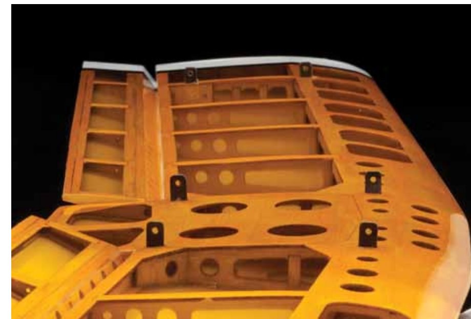
▲ This is the underside of the upper wing, showing the carbon tabs that are built into the wing, forming the attachment points for the cabanes and wing struts.
