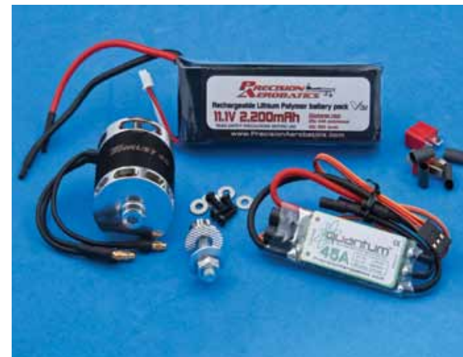
The main components of the power system are the Thrust 40 brushless outrunner motor, Quantum 45-amp ESC, and 2200-mAh 3-cell LiPo battery. The propeller adapter and Deans connectors are also part of the iPA's system.
