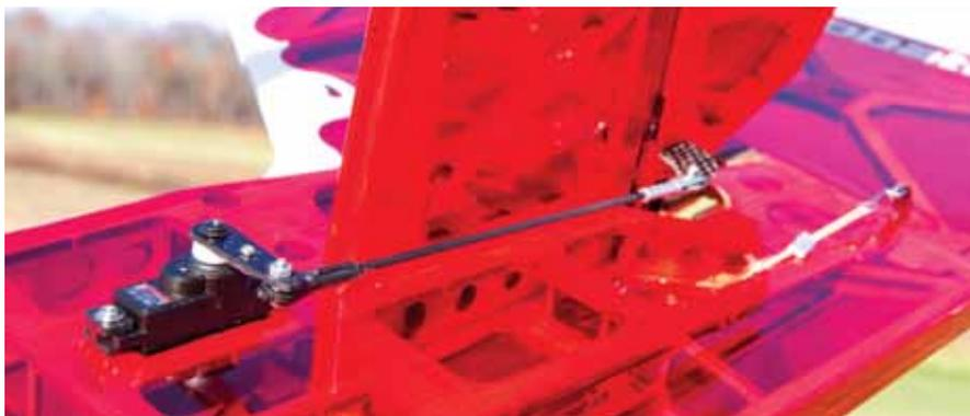
The hardware includes German-made ball links and CNC-machined clevises.
