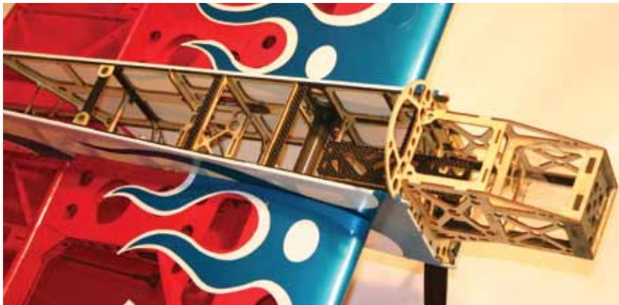
The Addiction X's FiberFusion construction method is exclusive to Precision Aerobatics airplanes. It combines carbon fiber, balsa and ply to produce a lighter, stronger and more rigid aircraft.
